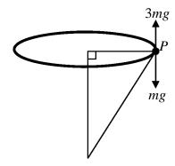
A model aircraft P, of mass  $m = 8 \,\mathrm{kg}$  is attached to the end of a 10 m long inelastic wire, with the other end fixed to the ground.
