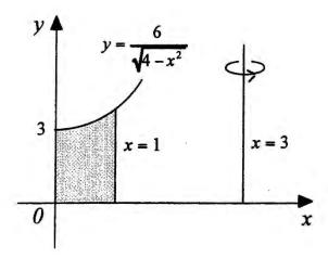
A mould for a section of concrete piping is made by rotating the region bounded by the curve  $y = \frac{6}{\sqrt{4-x^2}}$  and the *x* axis between the lines x = 0 and x = 1 through one complete revolution about the line x = 3. All measurements are in metres.
